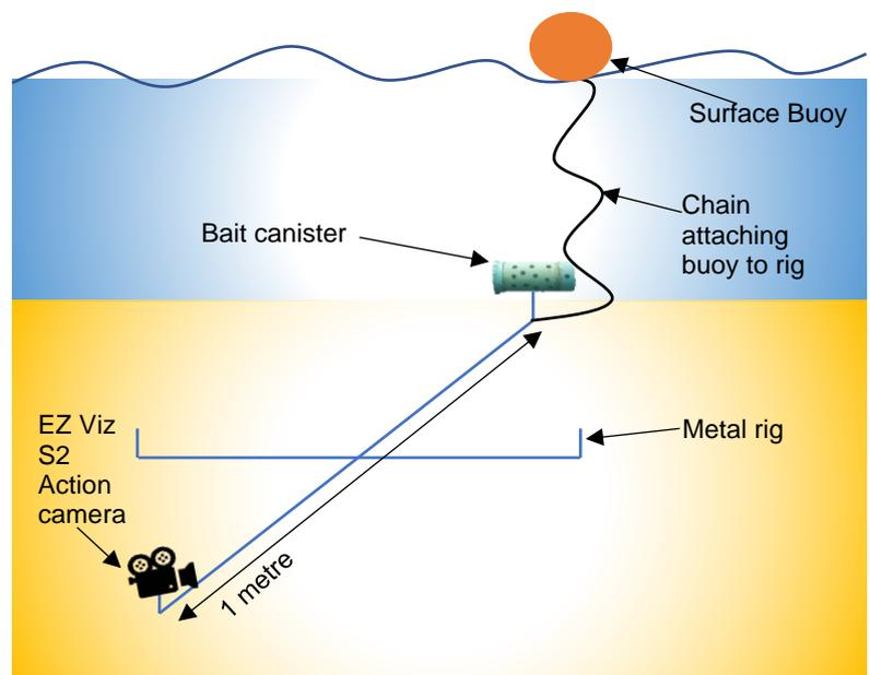
Figure 3. Diagram created using Microsoft Word to depict how the BRUV rig was set up during deployments.
